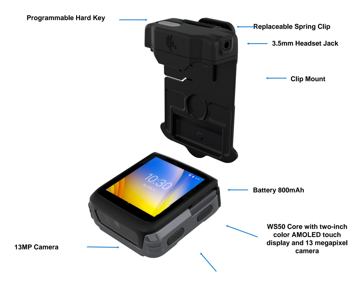
Replaceable Protective Shell with four hard keys
